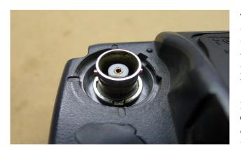
I found an O-ring that fit the approximately 5/16" diameter of the BNC connector at the local hardware store. I slipped it over the BNC and tamped it down to
